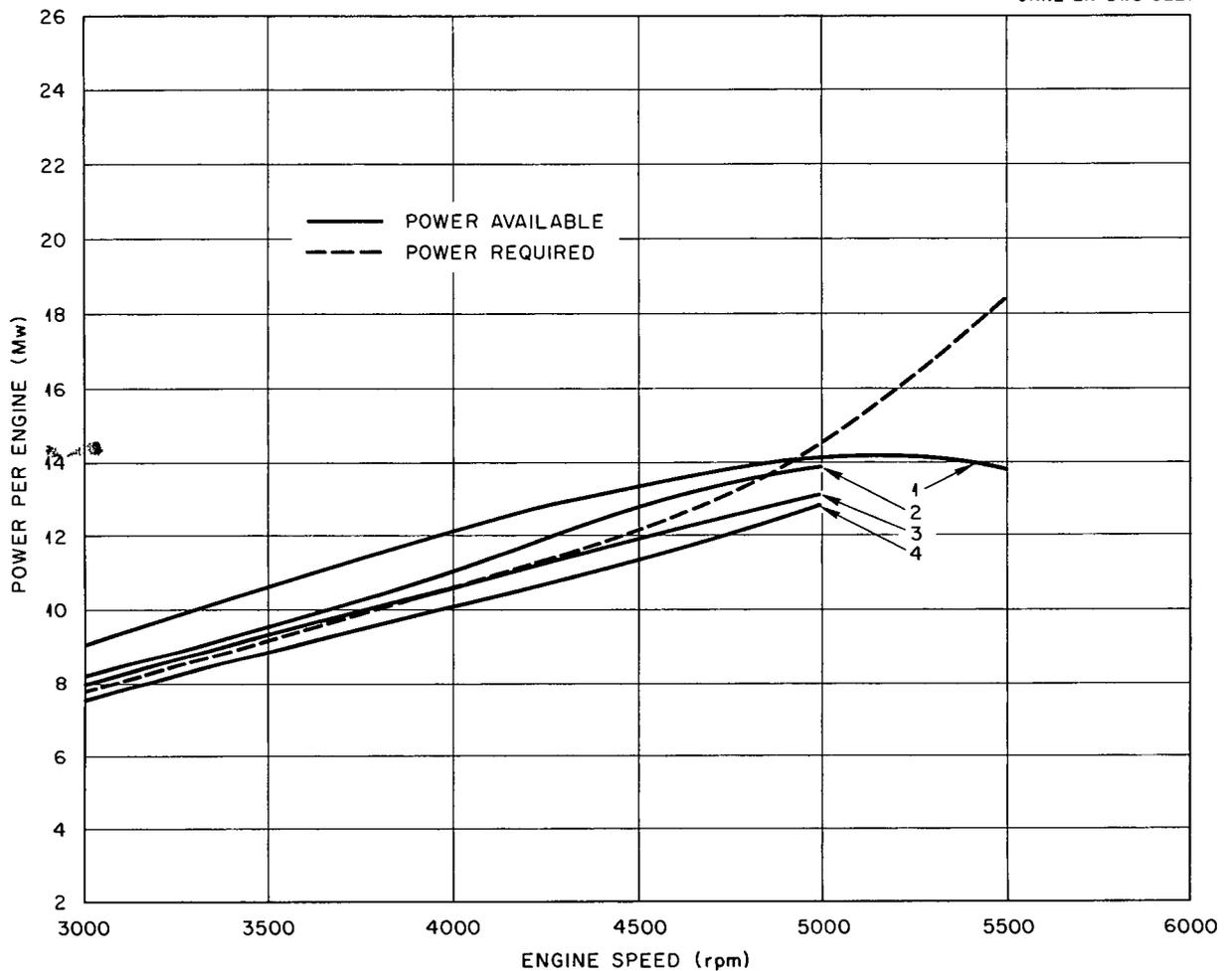
**Fig. 23 Steady State Power Delivered with 60% NaK Bypassed Steady State Engine Power Required vs Engine Rotor Speed** (1) Pump speeds constant at rated values (2) NaK pump speeds constant fuel pumps engine-driven (3) fuel pump speeds constant NaK pumps engine driven (4) fuel and NaK pumps engine driven
