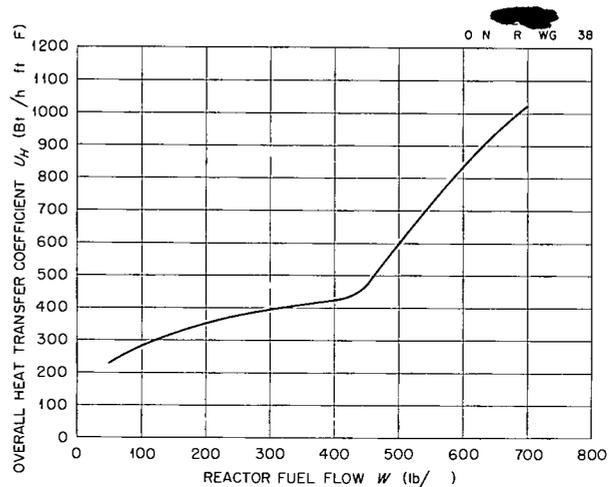
Fig 1 Variation of the Over All Heat Transfer Coefficient of the Main Heat Exchanger with Reactor Fuel Flow. Mean temperature 1450°F NaK flow 320 lb/sec
