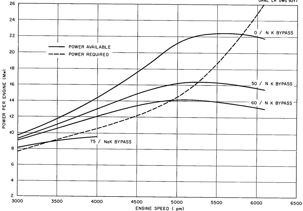
**Fig 19 Steady State Power Delivered with NaK Bypass Percentage Constant Steady State Engine Power Required vs Engine Rotor Speed Reactor and four Allison J 71 engines at SL static conditions exhaust nozzle open fuel and NaK pump speeds constant at rated values**
