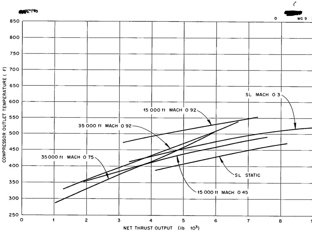
**Fig 5 Variation of the Steady State Compressor Outlet Temperature with Net Thrust Output for the G-E X 61 Engine Exhaust nozzle open**
